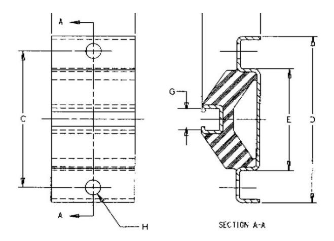
Lord Machinery Mounts are designed to support heavy equipment and isolate intermittent or continuous vibration.
