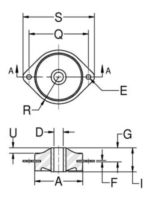
Lord Plateform Mounts provide effective isolation against vibration. The contour of the flexing element was developed to provide uniform stress distribution. This, plus high strength bonding and the use of specially compounded elastomers, provides maximum service life.
