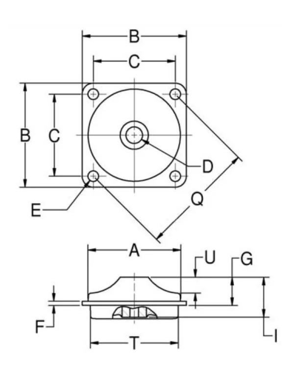
These versatile mounts are available in three types, each type featuring square, diamond or holder configurations to suit a variety of design requirements. The three types, Plateform Mounts, Heavy-Duty Plateform Mounts and Multiplane Mounts, offer a range in load ratings from 0.5 to 600 pounds.
