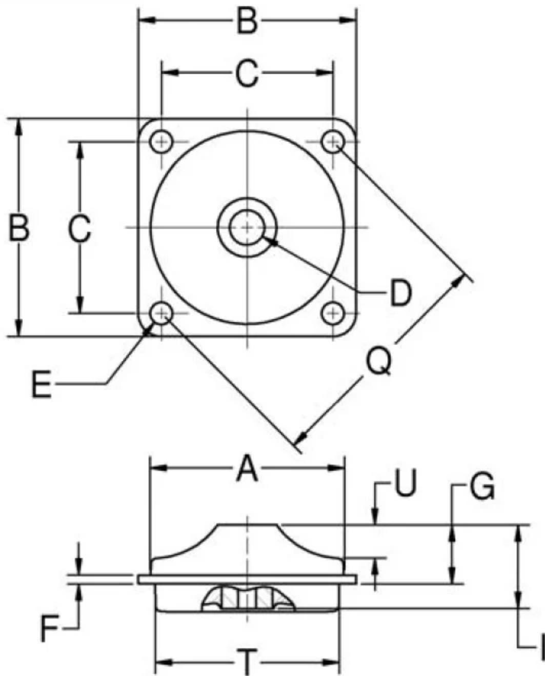
These versatile mounts are available in three types, each type featuring square, diamond or holder configurations to suit a variety of design requirements. The three types, Plateform Mounts, Heavy-Duty Plateform Mounts and Multiplane Mounts, offer a range in load ratings from 0.5 to 600 pounds.
