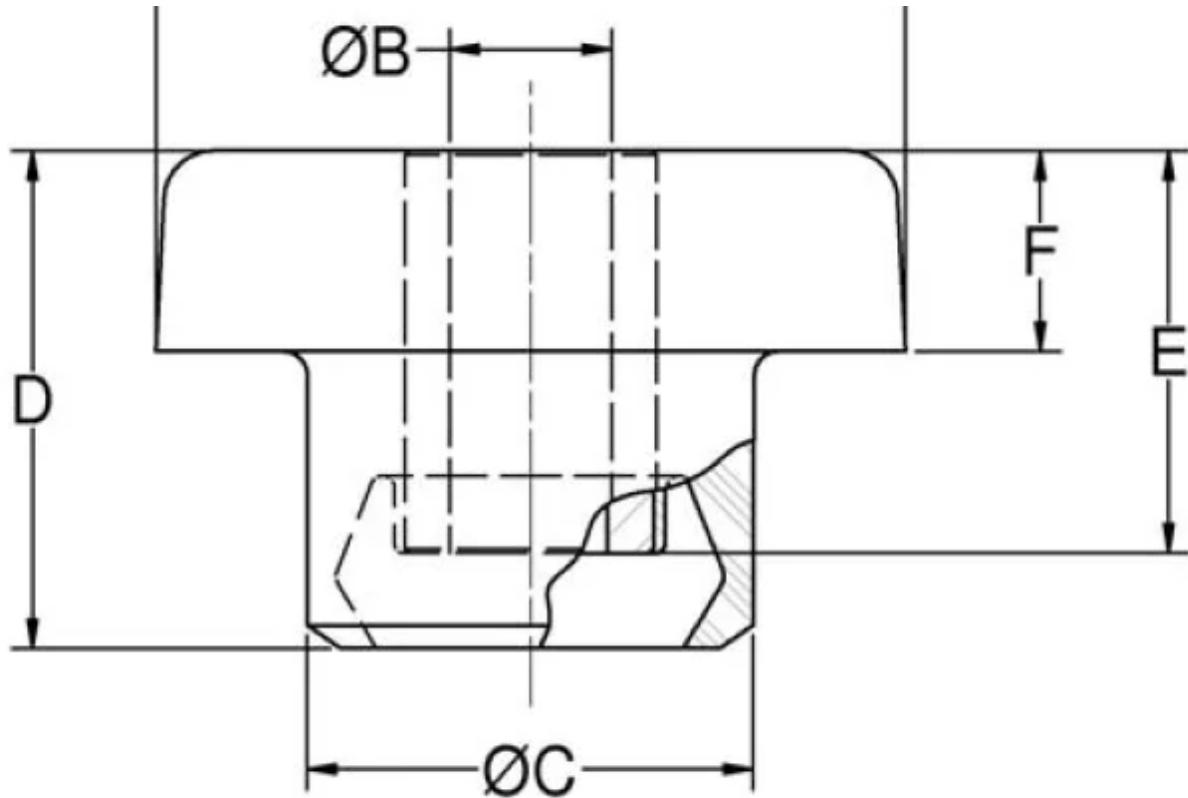
Center Bonded Mounts isolate vibration, control shock and reduce noise due to structure borne vibrations. Available in a full range of rated load capacities and able to withstand shock loads of 10 g's, these mounts effectively protect equipment and improve operator comfort. They are ideal for automotive, marine, railroad and industrial markets.
