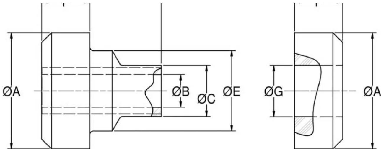
Two-Piece Mounts are designed for applications involving severe dynamic forces in the static load direction, as well as the rebound direction. Travel is limited in both directions by rubber in compression which provides snubbing.
