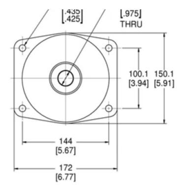
Conical mounts from Lord Corporation provide effective vibration isolation and noise attenuation with a simple, robust mount design. Consistent performance, high load bearing capabilities and a choice of radial stiffness characteristics are key features of these mounts. For more demanding vibration and noise reduction requirements, Lord integrates conical mounts with surface-effect technology to form an advanced control solution known as Hystec™ Systems.
