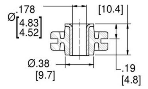
Lord Grommet Isolators provide effective, economical vibration isolation for light loads. They are suitable for commercial and military applications including computers, disk drives, business machines, precision instrumentation and general industrial equipment.
