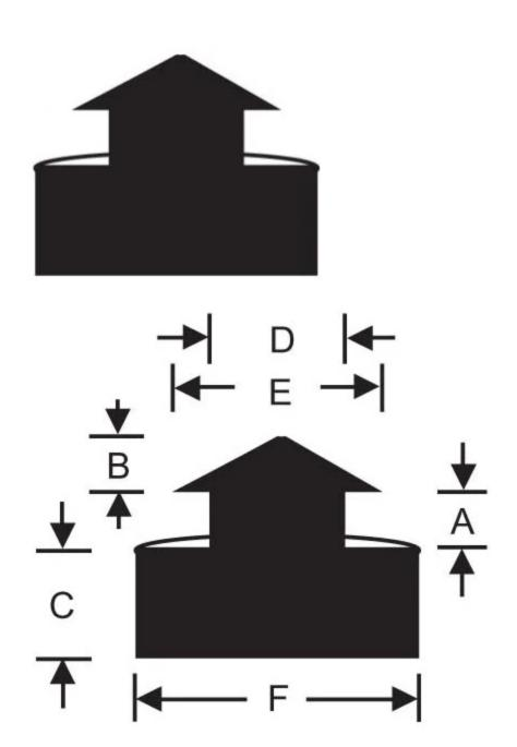
RPM's rubber recessed bumpers are used to protect doors or truck bodies from damage. They are also used as feet for large vibrating equipment.
