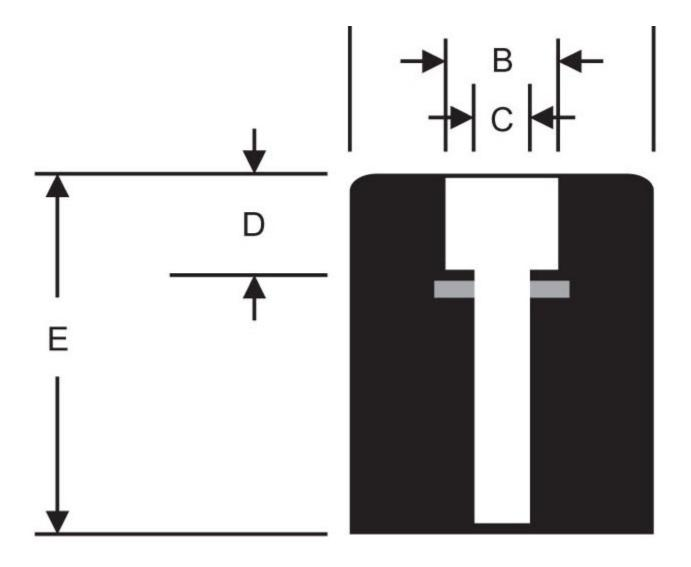
RPM's rubber recessed bumpers are used to protect doors or truck bodies from damage. They are also used as feet for large vibrating equipment.
