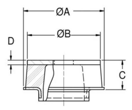
Two-Piece Mounts are designed for applications involving severe dynamic forces in the static load direction, as well as the rebound direction. Travel is limited in both directions by rubber in compression which provides snubbing.
