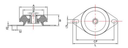
Flange mounts, or anti-vibration mounts, are universal mounting and popular in a wide range of applications and industries. Flange mounts are cost-effective, high-performing, and easy to install. The rubber is used in shear compression providing optimum performance and a wide range of flexibility. Offering vibration reduction up to 95%.
