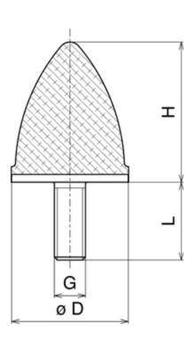
RPM Mechanical's vibration Buffer isolator's are designed to protect structures and equipment from impact forces.† They are usually fitted as non-metallic stops or incorported in vehicle suspension systems to provide progressive stiffening under increasing load.
