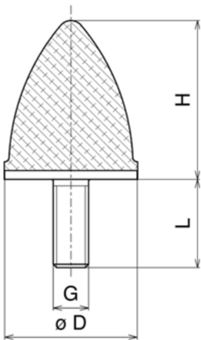
RPM Mechanical's vibration Buffer isolator's are designed to protect structures and equipment from impact forces. They are usually fitted as non-metallic stops or incorporated in vehicle suspension systems to provide progressive stiffening under increasing load.
